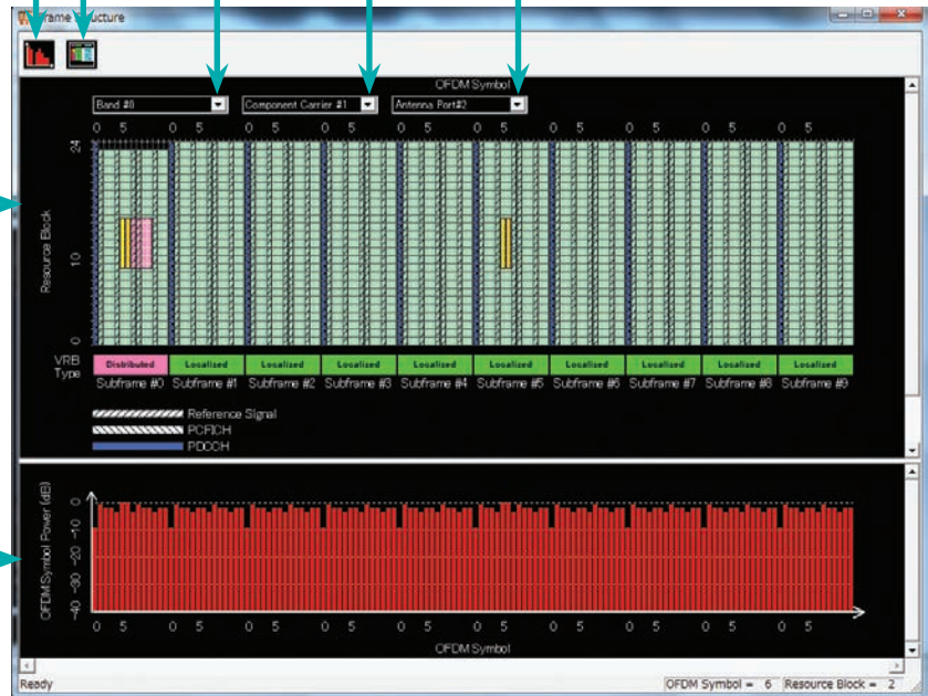
Frame Structure Screen (LTE-Advanced)
